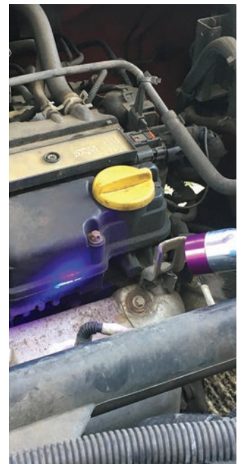
...there is the leak
